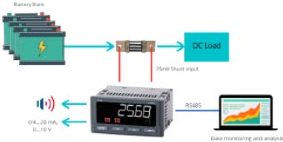
Fig. 1 - Possible setup for Battery System monitoring
