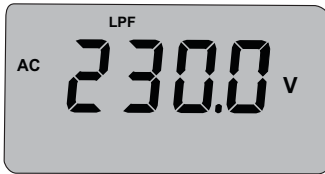
Fig 8.2 Low Pass Filter mode
