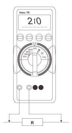
During Insulation resistance measurement the ON symbol flashes as long as the high voltage is present at the terminals
