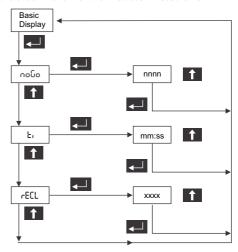
Structure of command menu for Resistance & Continuity measurement
