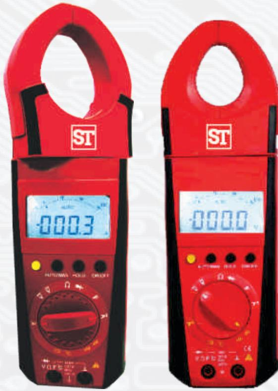
**Delta 1000/300** measures important electrical parameters like AC Current (TRMS), DC Current, AC Voltage(TRMS), and DC Voltage. It also features Capacitance, Ohm & Continuity, frequency, and Duty cycle and temperature measurement.
