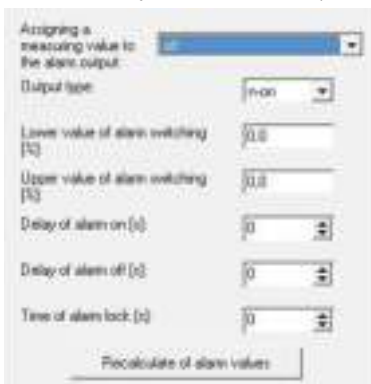
Fig. 13. View of the alarm configuration window.
