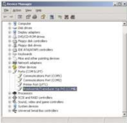
Fig. 8. View of the device manager window together with the installed P43 transducer, which the port COM6 is assigned to.
