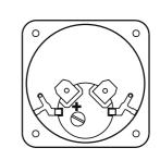
This is available as a rear mounted factory fitted option. The unit contains a Ø 6mm 'festoon' style lamp available in 6V, 12V or 24V. Please contact the sales office for more
