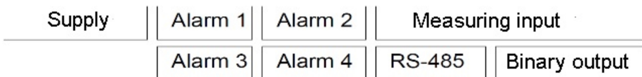
Fig. 4: Galvanic isolation of the N32H meter.
