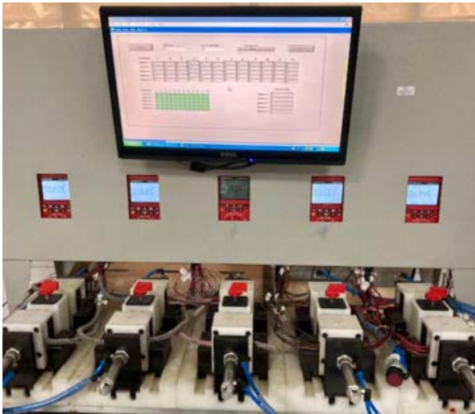
Automated test bench for product testing using Sifam Tinsley multimeter's as reference source
