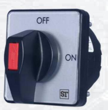
**EPSILON CAM SPRING RETURN SERIES** provide contacts that are held closed only when the switch is turned against the mechanism spring. The mechanism returning the contacts to their original state upon release of the actuator. This type of switches are known as "Momentary switches".
