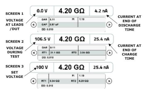
• You can save the data of this test by pressing the button. After pressing this button a message will appear to tell you about the file number. You can press the OK button on the message box in order to go back to the measurement screen.
