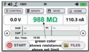
The go no go setting is also available in the voltage mode where the voltage text color will turn red if the go no go setting is ON and the voltage is above the decided limit
