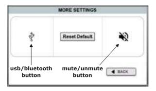
**Communication interface setting:** This meter has 2 interfaces for communication (Bluetooth or USB). Please note that at any given time only one interface can be used for communication. To select which interface to use you can press the USB/bluetooth button in the more settings window. The currently activated interface is shown by the icon of this button.
