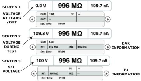
• You can save the data of this test by pressing the button. After pressing this button a message will appear to tell you about the file number. You can press the OK button on the message box in order to go back to the measurement screen.
