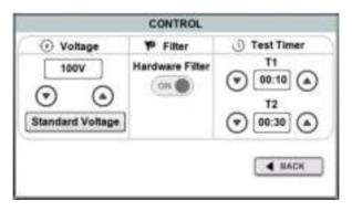
Here you can set the voltage using the voltage up and down in steps of 10V below 1000V and in steps of 25V above 1000V. There is also a standard voltage button to set standard testing voltages (100V, 250V, 500V, 1000V, 2500V, 5000V).
