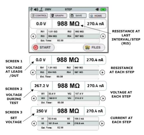
Please note that in step mode if the meter is running on battery supply, the meter will not be able to deliver 5000V to a load resistance of below  $10 \text{ M}\Omega$ .
