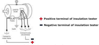
Insulation resistance testing of motor
