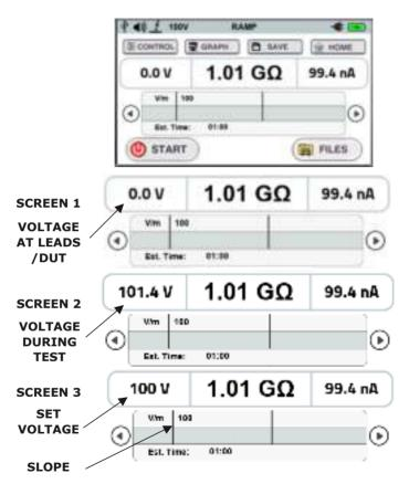
You can save the data of this test by pressing the button. After pressing this button a message will appear to tell you about the file number. You can press the OK button on the message box in order to go back to the measurement screen.
