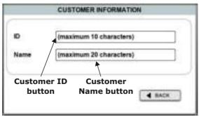
In this window you can edit the customer ID and name by clicking on their respective buttons. Then an alphanumeric keyboard will appear where you have to enter the customer ID/ name and then press the <code>ENTER</code> key.
