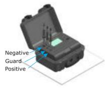
• Then push the probes into the meter and rotate the probe rotor as shown below so that the probe gets locked to the meter.
