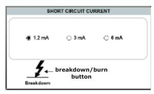
You can select the desired short circuit current by clicking on the corresponding button. And you can change the breakdown/burn setting by clicking on the icon in the bottom left corner which indicates the present breakdown/burn setting.
