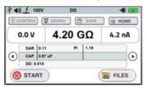
Because there are a lot of parameters to be displayed they have been divided into three sub screens which can be scrolled using the scrolling arrows. Figure shows the sequence of the screens along with the parameters displayed on the corresponding screen.
