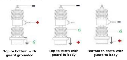
+ Positive terminal of insulation tester - Negative terminal of insulation tester
