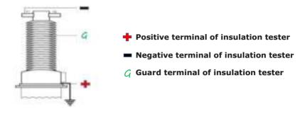
Primary to ground with body of the CT connected to guard
