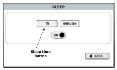
Here you can change the sleep time by pressing on the minutes button and a keyboard will appear where you have to enter the minutes and press obtain. The sleep mode can also be turned ON/OFF by clicking on the ON/OFF button.
